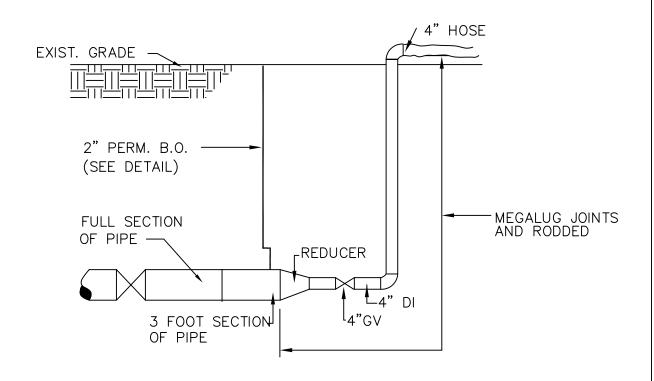
AFTER THE COMPLETION OF THE FINAL FLUSHING THE CONTRACTOR SHALL REMOVE THE TEMPORARY FLUSHING CONNECTION AND INSTALL A CAP WITH MEGALUGS AND A THRUST BLOCK
